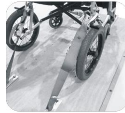
Fitting the rear restraint
