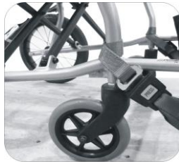
Fitting the front restraint
